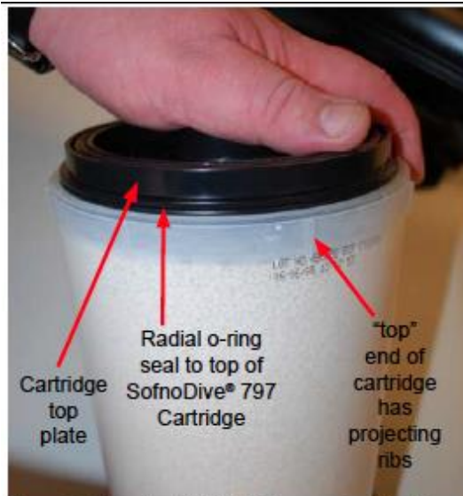
Figure 1-23. Loading the MkVI Discovery Cartridge Top Cap into the replacement SofnoDive® 797 cartridge
